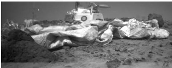
Figure 8. Inflated membrane structure — Mars Pathfinder landing gasbags (courtesy of NASA)
