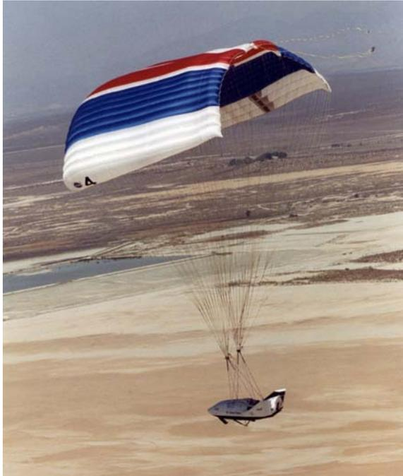
Figure 7. Parafoil to slow descent of experimental spacecraft
