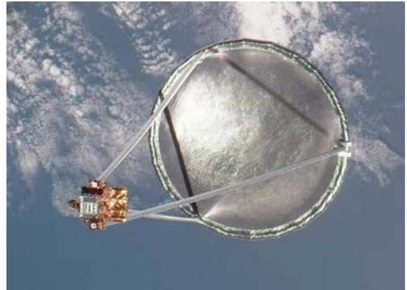
Figure 5. Inflatible antenna experiment (IAE)
